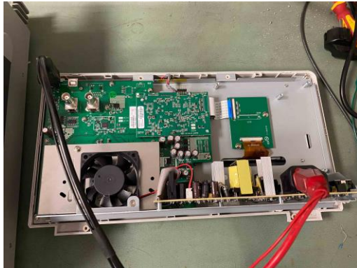
Measurements between power plug-in GND and enclosure.
